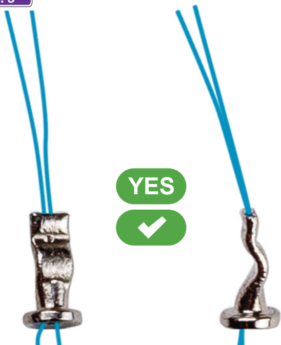
FIG. 5 Front and side enlarged views of a correctly crimped fastener
